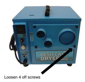
Rotate duct plate
