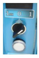
RH control – fit the RH sensor into connector located on the front panel and turn on/off switch to **1** RH, the TD3000 will now be controlled by the remote RH sensor to prevent possible over drying.
